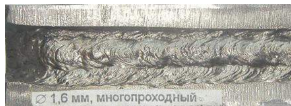
Fig.4. Formation of metal of multilayer weld
