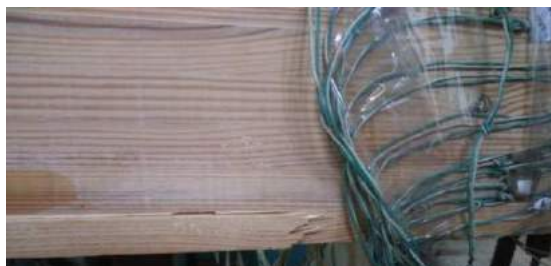
Fig.4. Fracture of the GLB-3
