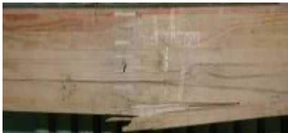
Fig.3. Fracture of the GLB-1
