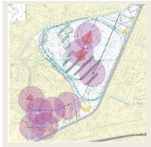
Fig.2. A fragment of a planning scheme of location of the primary waste collection points with the definition of their influence zone on the example of a residential area in Kyiv
